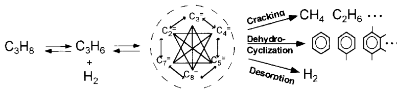
Scheme 1. Reactions of propane on H-ZSM5-based catalysts.
